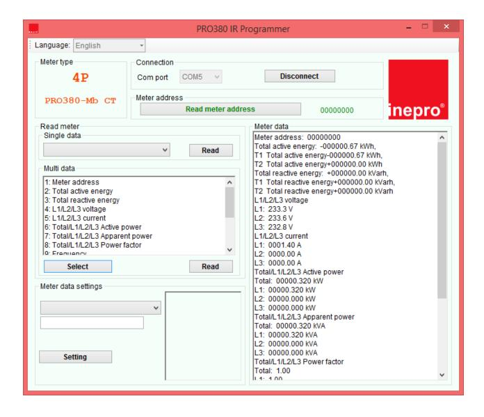
Start the program and select the COM port. Press "CONNECT" and "READ METER ADDRESS". The software will now communicate with the meter and the METER TYPE and METER ADDRESS are filled in if this is received back from the meter.
